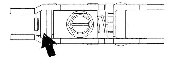
4. Following torque link replacement repeat step 2. The control rack must return to idle rack positon.
